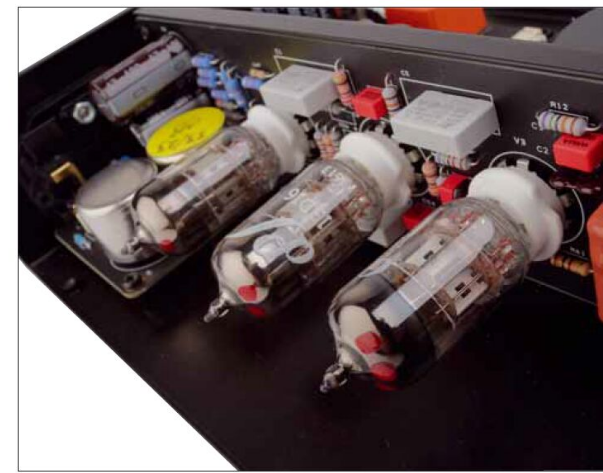
And this is the version with the standard tubes and the 40-ohm MC transformers for high-impedance cartridges
