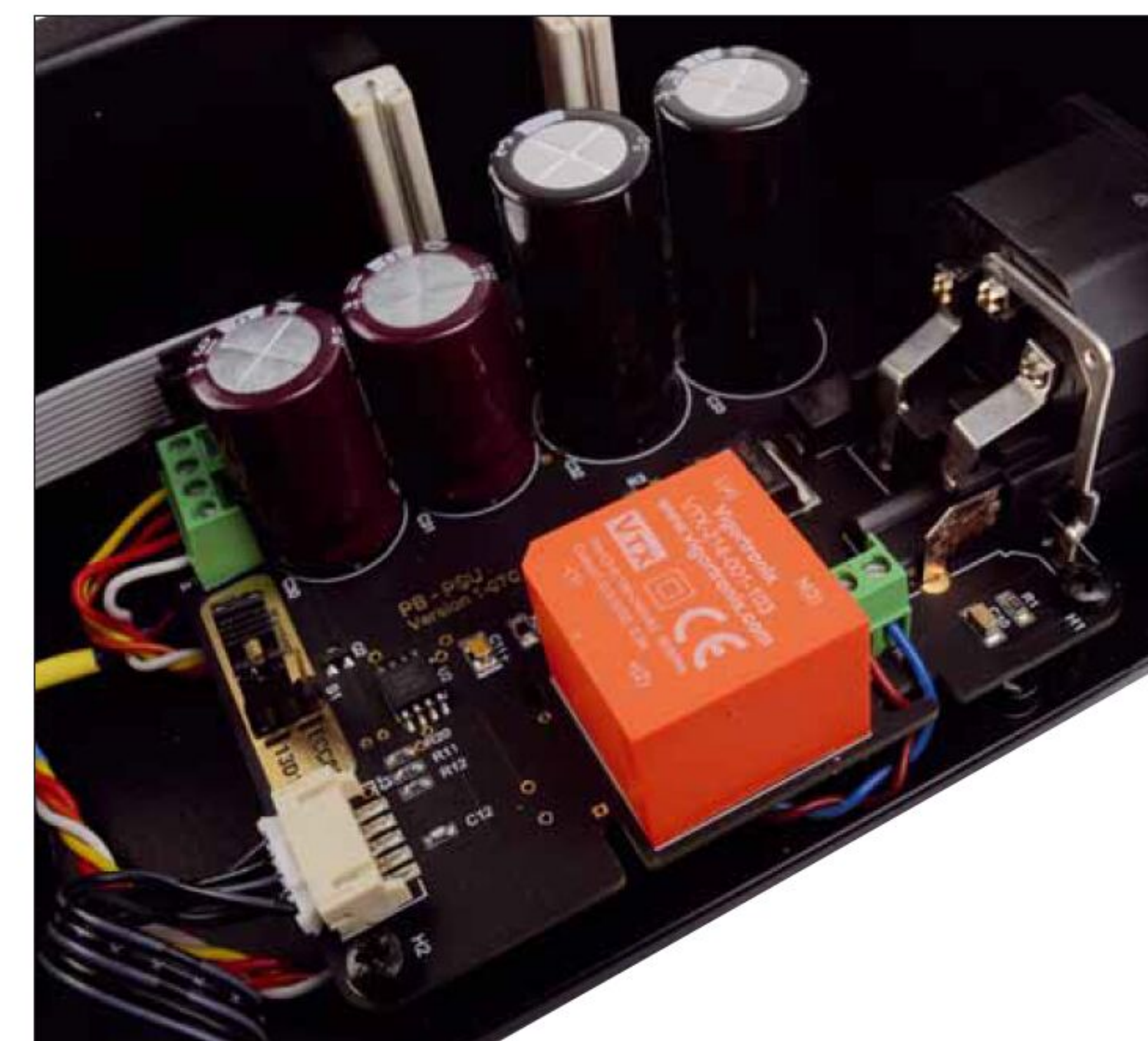
The input board with mains filter, screening, and jumper. This is much better made today than it used to be
